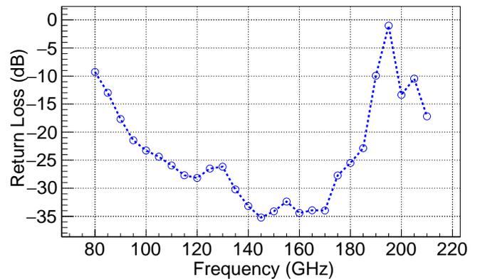
Fig. 2. Return Loss of a broadband horn.
