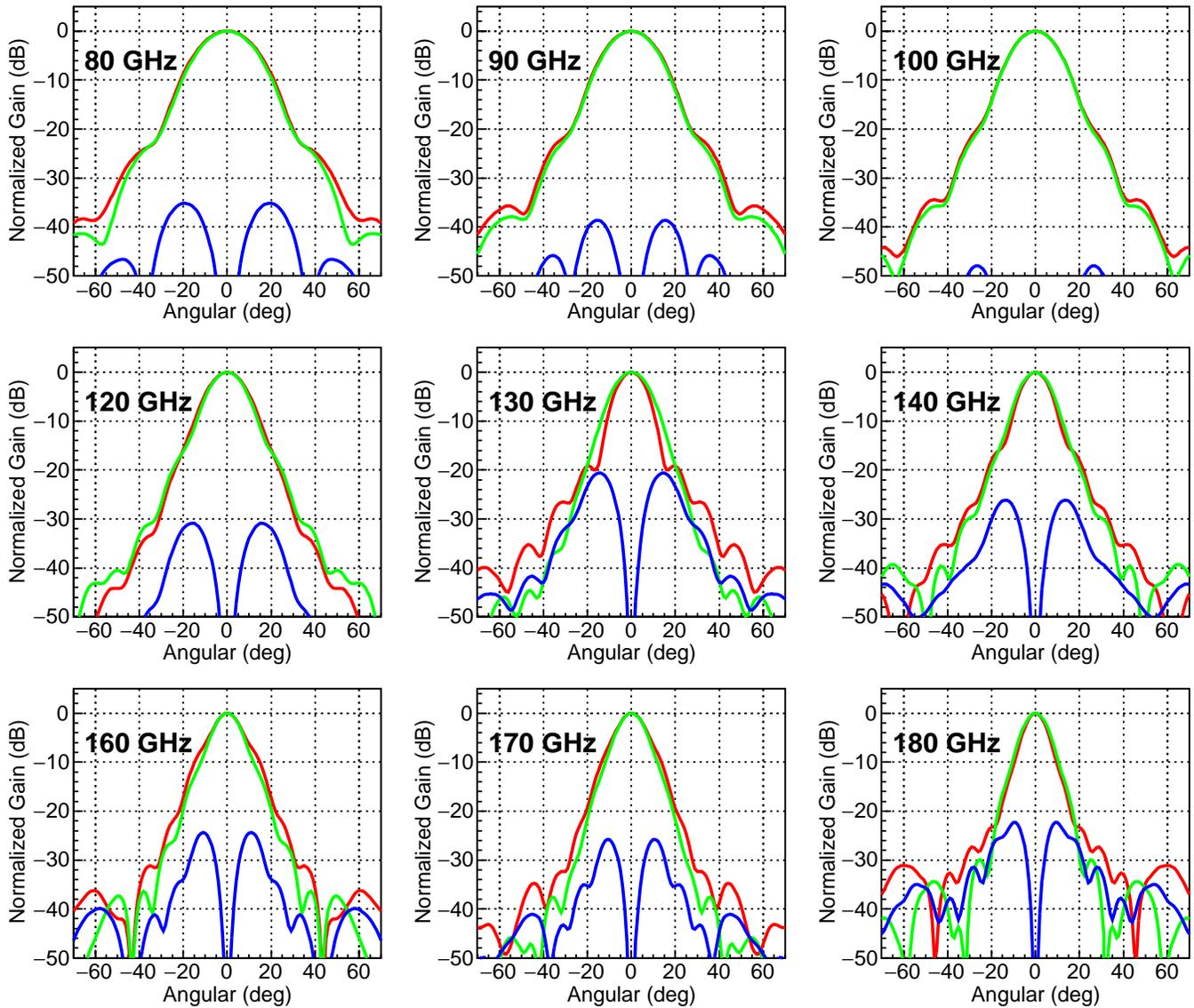
Fig. 3. Simulated beam pattern of an 80 - 180 GHz horn. Green, red and blue lines are E-plane and H-plane of Co-polarization and Cross-polar diagonal plane, respectively.
