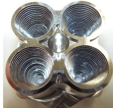
Fig. 4. 4 pixel 80 - 180 GHz horn array.
