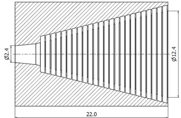
Fig. 1. Cross-section of a broadband corrugated horn. The unit of length is millimeter.
