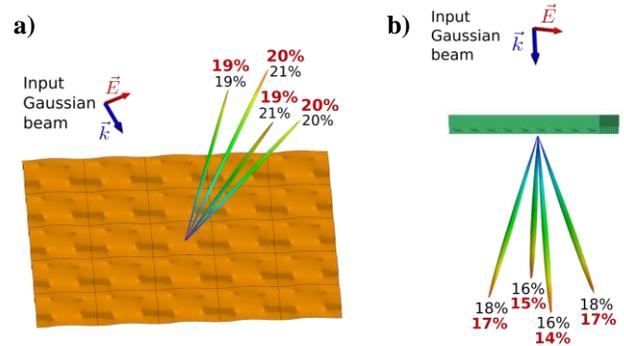
Fig. 4 Far-field beam intensities measured (in red) and compared to the simulation results, in reflection (a) and in transmission (b).
