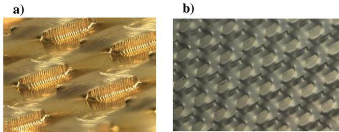
Fig. 3 Pictures of the manufactured (a) reflective and (b) transmissive gratings taken with a microscope.
