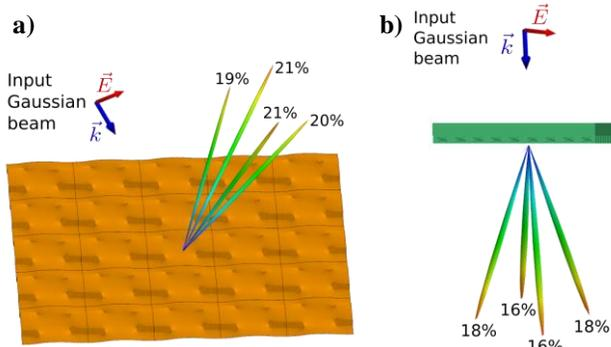
Fig. 2 Far-field beam patterns calculated by the electromagnetic simulations in reflection (a) and in transmission (b).
