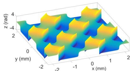
Fig. 1 Phase grating profile calculated by the iterative algorithm.
