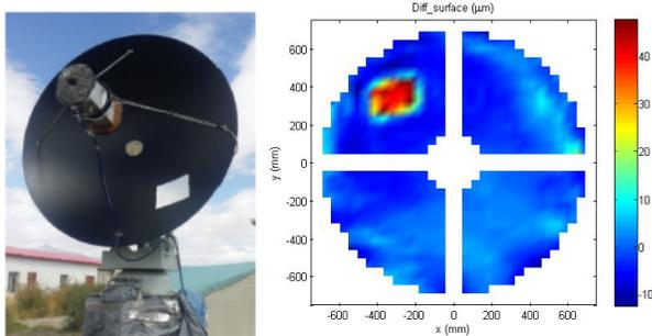
Fig. 11 Surface profile measured with two layers of foil
