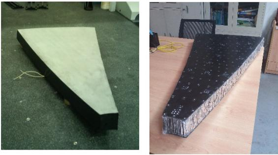
Fig. 5 The CFRP prototype panels. Left: with side seal, right: without side seal.
