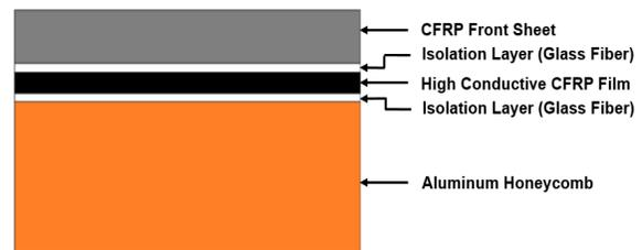
Fig. 7 De-icing system of CFRP panel.
