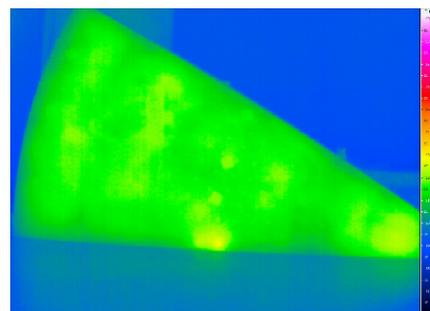
Fig. 9 Temperature distribution of CFRP panel for a input heat flux of 45W/m<sup>2</sup>.
