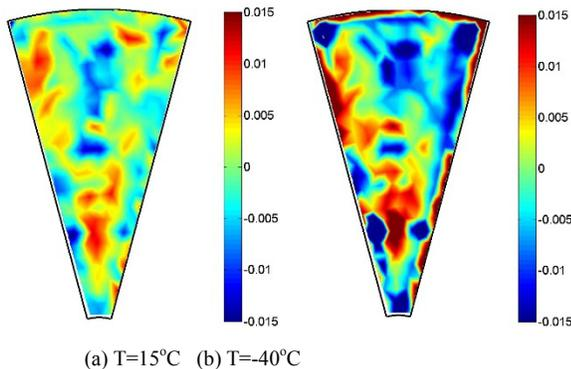
Fig. 6 Residual surface error for Panel A after best fitting with a parabolic surface.
