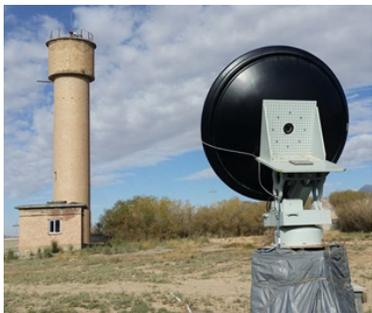
Fig. 10 Experimental setup of the near-field holographic measurement
