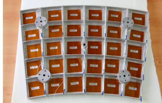
Fig. 3 Aluminum panel anti-icing system.
