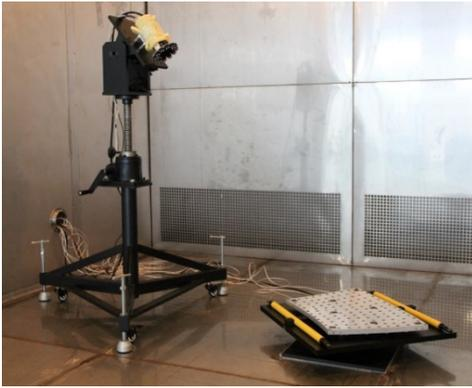
Fig. 2 Experimental setup of the photogrammetry measurement in a climate chamber.
