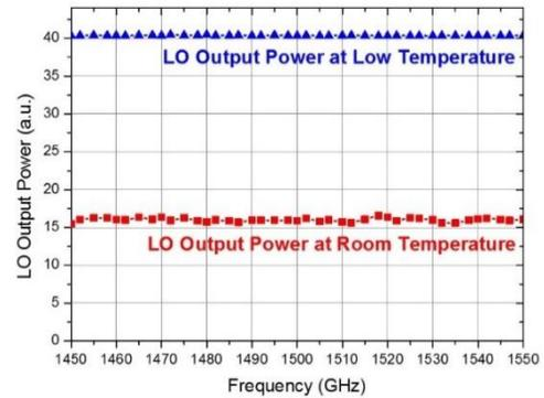
Fig. 7 The LO output power measurement at room temperature and low temperature.
