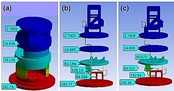
Fig. 6 (a) The simulated temperature distribution of the bare cartridge. (b) The simulated temperature distribution when the synthesizer is turned off. (c) The simulated temperature distribution when the synthesizer is turned on.
