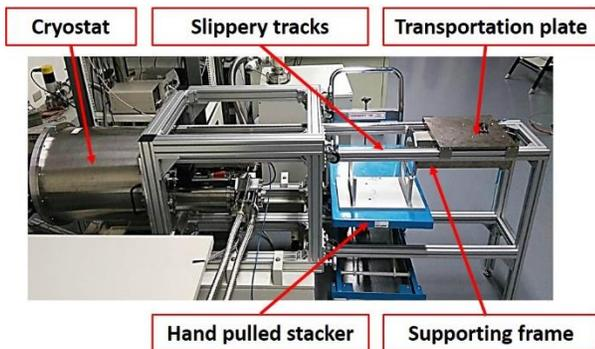
Fig. 3 The loading system and testing cryostat for cartridge.
