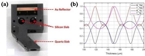
Fig. 2 (a) The four-pixel power distributor module. (b) The calculated transmittance and reflectance of polarizing beam splitters versus thickness.
