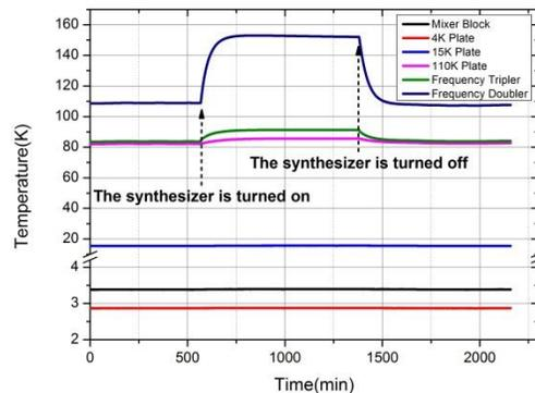
Fig. 5 The temperature distribution of the cold cartridge.
