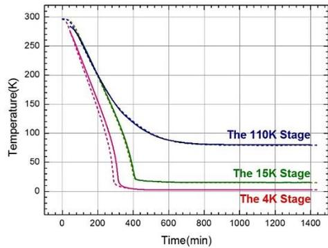
Fig. 4 The temperatures of the three cooled stages versus time during cooling procedure. The dashed line is the result of the bare cartridge, and the solid line is that of the engineering model cartridge.
