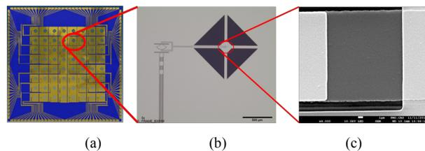
Fig. 1 (a) 8x8 superconducting Ti transition edge sensor array. (b) photo of the microbridge integrated with twin-slot antenna via CPW transmission line. (c) Ti microbridge with dimension of 16 $\mu$ m x 16 $\mu$ m.
