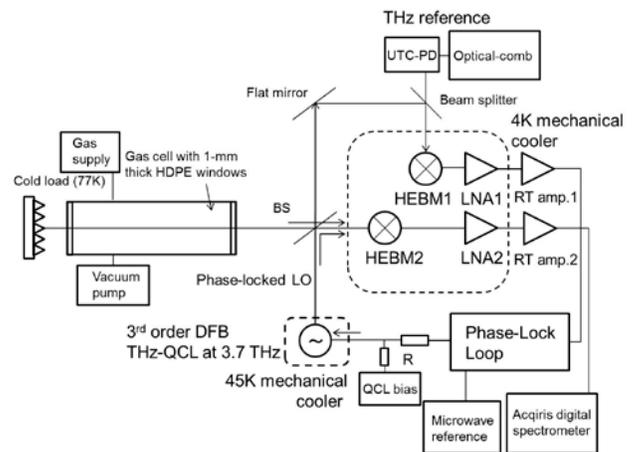
Fig. 1. A gas cell system for the measurement of emission line spectra of molecules using an HEBM with a phase-locked THz-QCL-HEBM. A 3<sup>rd</sup> order DFB THz-QCL at 3.7 THz was phase locked using an HEBM1 to a THz reference, which was generated by an optical comb and a UTC-PD. The phase-locked THz signal was fed into another HEBM2 using a beam splitter. The line spectra were obtained using a digital spectrometer with a bandwidth of 1 GHz and 13 K channels.
