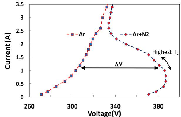
Fig. 1. Current-voltage characteristic of the Nb magnetron sputtering cathode using current stabilization in  $Ar/N_2$  and in pure argon gas mixture.
