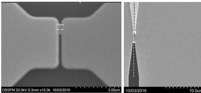
Fig. 7 Electron microscope picture of electrodes separated by a gap of ~100nm patterned by UV lithography. This is achieved when the arrows are misaligned by  $\Delta w$  (right picture).
