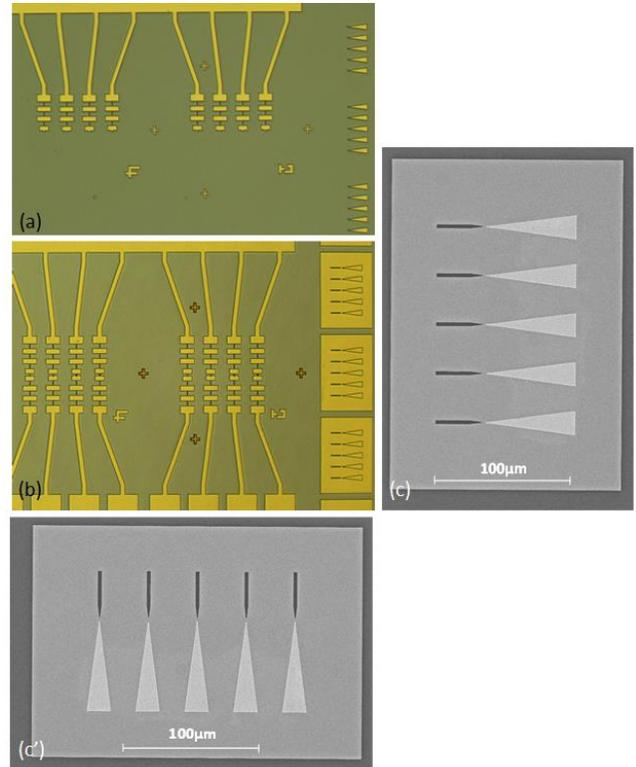
Fig. 5 Fabrication process sequence using standard 320nm UV lithography. (a) Definition of the first Au electrode, (b) definition of the second Au electrode which is closely and precisely aligned to the first one using horizontal and vertical arrow mark alignment.
