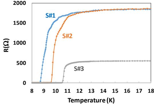
Fig. 2. Resistance versus temperature curves of ultrathin NbN films deposited on 3-inch Si substrates for a substrate temperature of 700°C during deposition. Critical temperatures are measured at the mid temperature transition. Using AFM technique and RIE end-point detection, the thickness is estimated to be 4-5 nm for films 1 and 2 and 6-7 nm for films 3.
