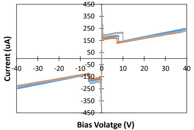
Fig. 8. First I-V curves of HEBs fabricated by UV lithography process using NbN layer with  $R_{\square} \approx 550 \Omega/\square$  and nanobridges of  $L \times w \approx 0.25 \times 2$ ,  $0.3 \times 2$  and  $0.4 \times 2 \mu\text{m}$ .
