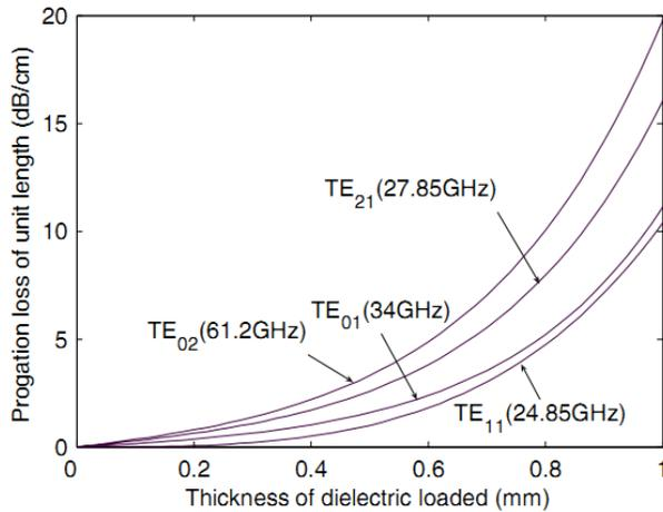
Fig. 4 Propagation loss of unit length vs. thickness of loss layer  $d=0.07$  cm (relative permittivity  $\xi''=11-j$ , waveguide radius  $r_w=0.56$ cm).
