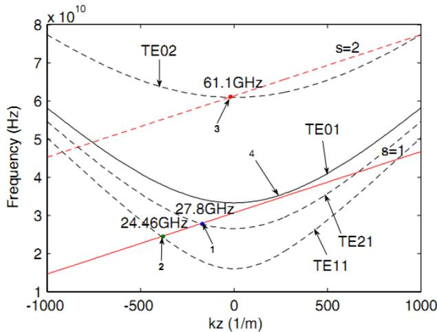
Fig. 3. Dispersion diagram of TE<sub>01</sub> gyro-TWT
