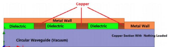
Fig. 1. Schematic view of the simulation model for gyro-TWT interaction structure.
