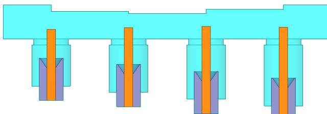
Figure 7.The equalizer structure by a series of resonance branches
