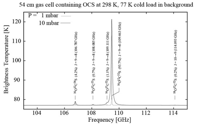
Fig. 5 Five lines show up across the CAMELS band in simulated OCS gas cell spectrum produced with the *am* radiative transfer code [7].
