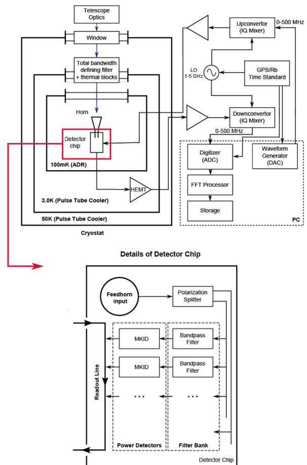
Fig. 1 System block diagram of the CAMELS instrument.
