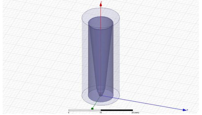
Fig. 3. HFSS model of the three-section MFA horn.
