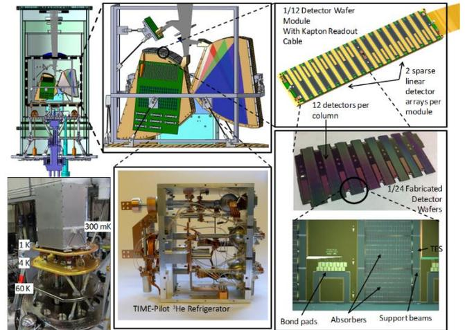
Fig. 1. TIME-Pilot instrument overview.
