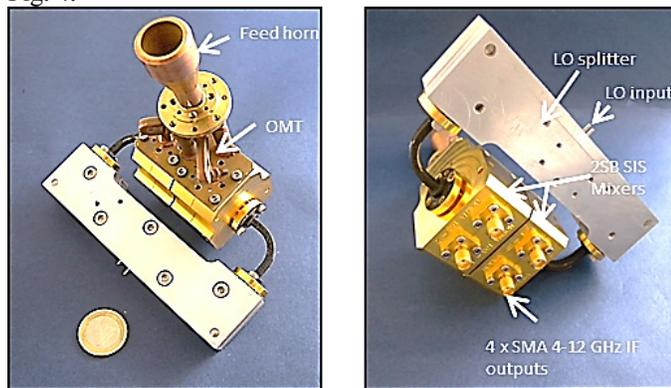
Fig.4: Views of the assembled 71-116GHz RF module.
