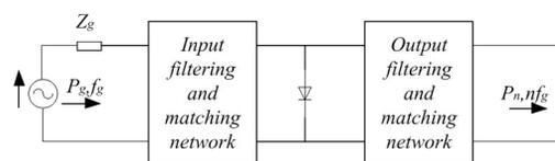
Fig. 1 The Schottky diode multiplier schematic diagram
