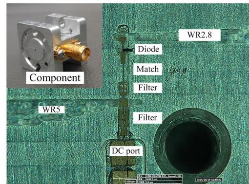
Fig. 5 Photograph and detail of 340GHz multiplier
