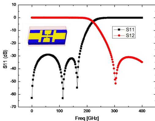
Fig. 4 simulation results and structure of CSMRs filter
