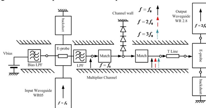
Fig. 2 Structure diagram of the 340GHz frequency doubler
