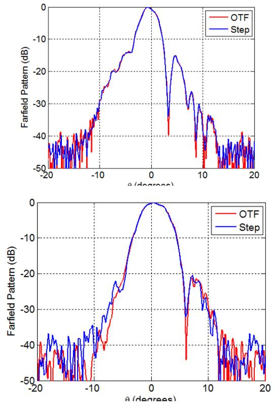
Fig.3 Far-field Comparison of OTF scan and Step-and-integrate scan. a) E-plane b) H-plane
