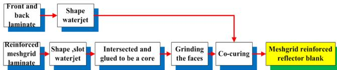
Fig. 3 Process flow of reflector blank
