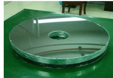
Fig. 8  $\Phi 500\text{mm}$  CFRP reflector completed
