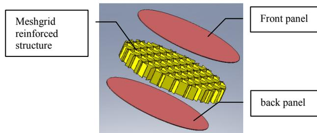
Fig. 1 CFRP reflector structure design
