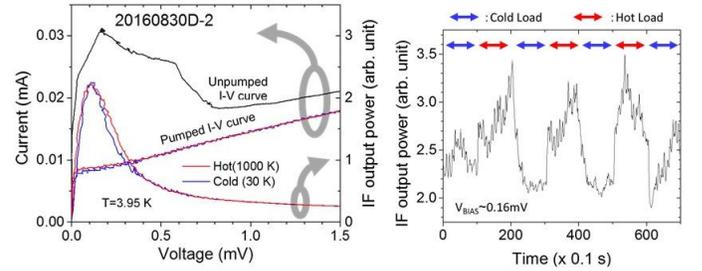
(a) I-V and IF output power characteristics (b) IF output power – Hot/Cold Loads
