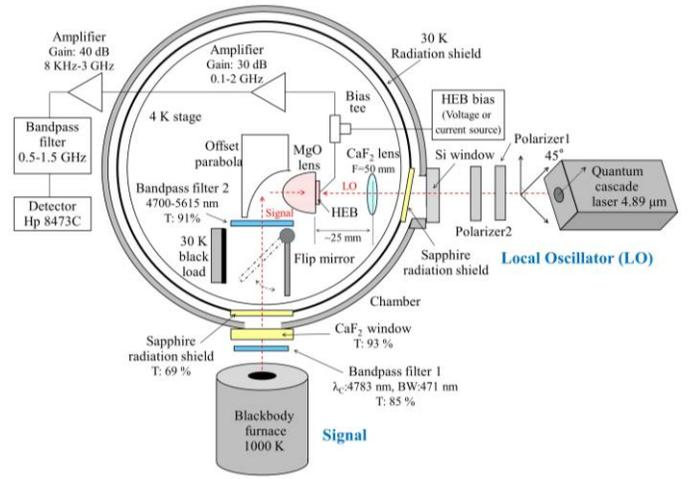
Fig. 4. Measurement setup for evaluating the MIR HEBs.
