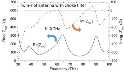
(b) Simulated impedance of the twin-slot nano-antenna at feeding point
