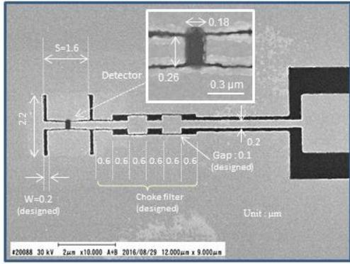
Fig. 3. SEM image of the MIR HEB,
