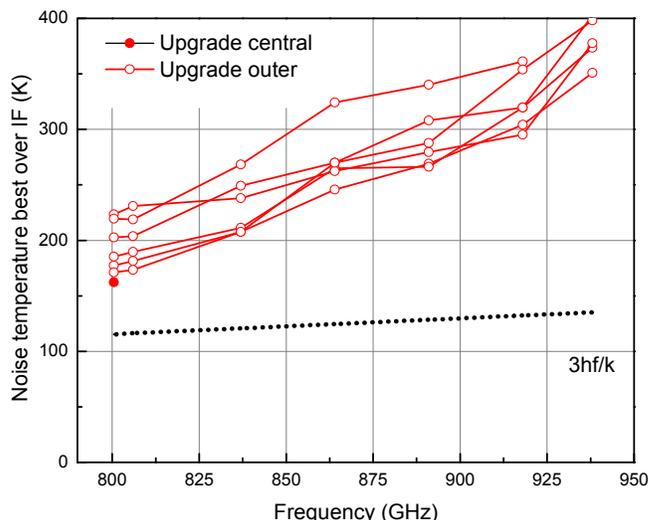
Fig. 7 Noise temperature at the best point in the IF band vs. for different LO frequencies. The data is corrected for the beam splitter as on Fig. 5. For the central pixel (solid dot) only the lowest frequency point was measured.
