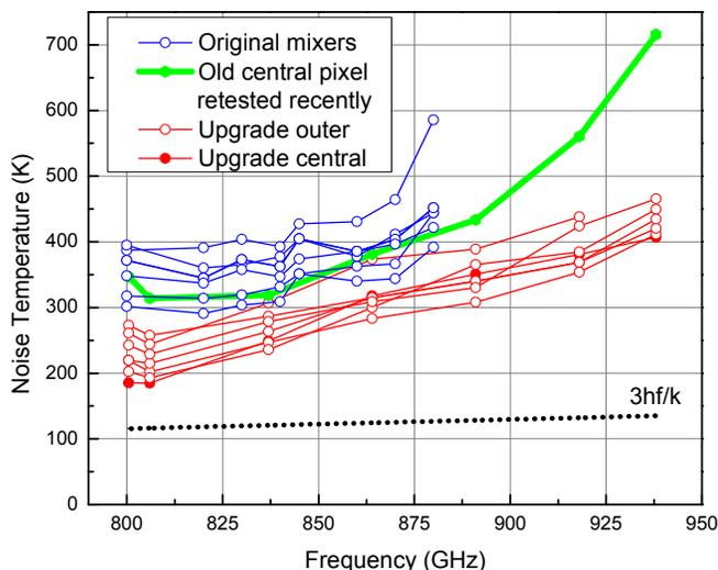
Fig. 5 DSB mixer noise temperature for the entire 4-12 GHz IF band vs. LO frequency. The noise temperature is corrected for about 10% insertion loss of a beamsplitter and for the hot LO (300K) contribution. The old mixers performances (blue curves), including additional recent verification for the central pixel (green curve), are compared here to results for the new mixers (red curves). For all the upgrade mixers the second minimum of the critical current suppression was used.
