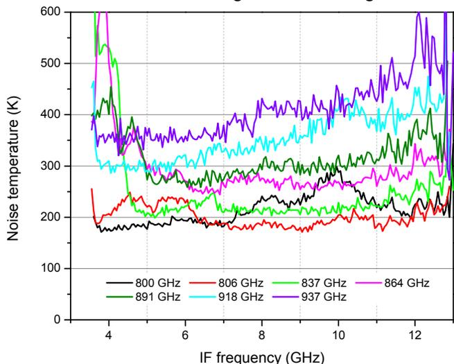
Fig. 6 Corrected noise temperature over the IF band for different LO points. Peaks are caused by LO noise and resonances in the testing horn. The presented lab data corresponds to one of the upgrade mixers installed later in an outer pixel of the array.
