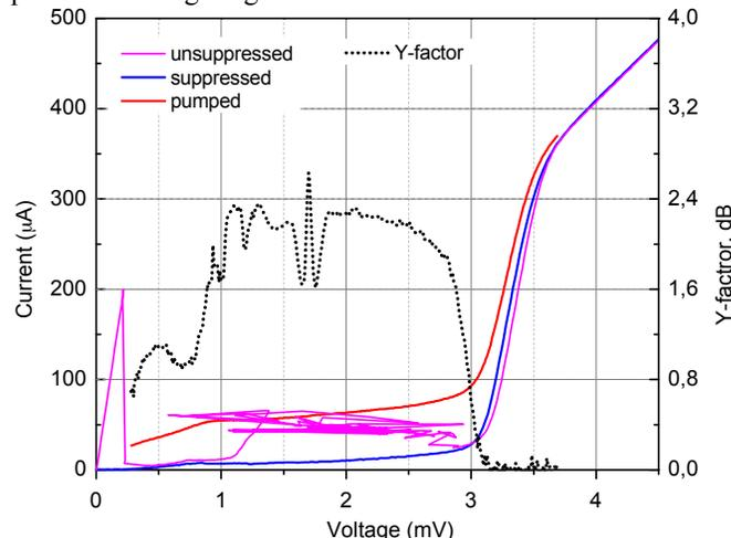
Fig. 8 IV-curves of one of the high band SIS junctions: autonomous unsuppressed (violet line), with suppressed critical current (blue line), pumped by LO signal providing an optimal noise temperature (red curve). The uncorrected Y-factor measured using 77 K/300 K loads is shown by dotted curve. The LO frequency is 800 GHz.
