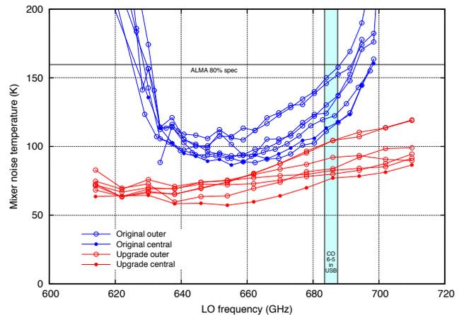
Fig. 1 DSB noise temperature of the new CHAMP+ low band mixers (red curves) compare to old ones (blue curves). Data is corrected for beam splitter insertion losses (5%). The curves with solid circles correspond to the central pixel of the array. The noise temperature in this figure is integrated over the entire 4–12 GHz IF band. Especially marked is the LO frequency range, where the CO  $j=6-5$  line (one of the prime goals of the band) appears in upped sideband of 4-8 GHz IF band.
