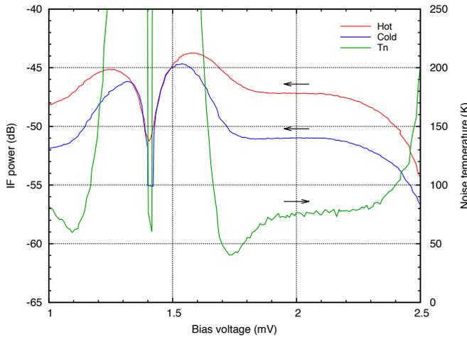
Fig. 3 Measured IF output power versus mixer bias voltage for hot (300K) and cold (77K) load – red and blue curves correspondingly. Using them, the noise temperature curve (green line) was calculated. Operating point is chosen close to 2 mV. The LO frequency is 650 GHz.
