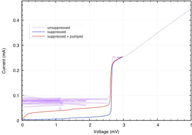
Fig. 2 IV-curves of the central pixel SIS mixer: unsuppressed (violet), with suppressed critical current (blue), with suppressed critical current and pumped by LO signal of 650 GHz (red).
