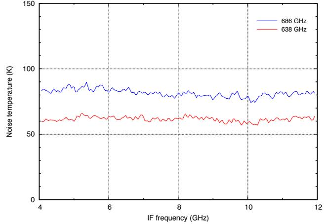
Fig. 4 IF noise temperature vs. frequency, measured for LO frequencies of 686 GHz (blue curve) and 638 GHz (red curve).
