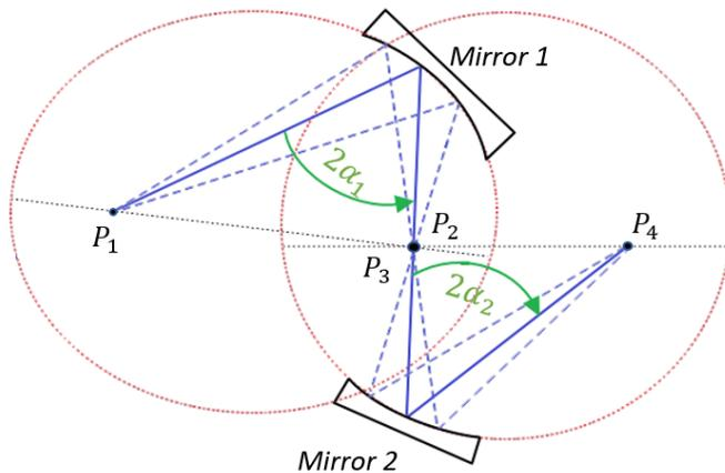
Figure.1 - Optical layout to minimize distortion using two elliptical mirrors. The main ray is represented by the blue solid line and the marginal rays are represented by the blue dashed lines. The point  $P_1, P_2, P_3, P_4$  correspond to focal points of the ellipse defined by the mirror 1 and 2 respectively.
