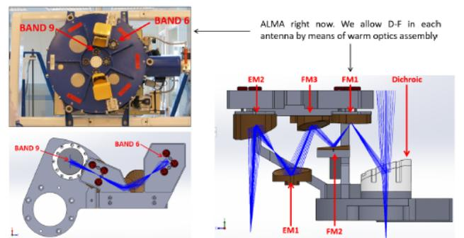
Fig. 5 Top view of ALMA cryostat (left top) showing the actual layout of the Bands. The left bottom image shows a top view of the support structure for the beam combiner assembly. A side view of the system is shown on the right side.
