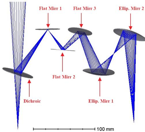
Fig. 3 Optical design of the beam combiner system made using Zemax software. The design has been made using a geometrical optical approximation by means of the Zemax sequential system option.
