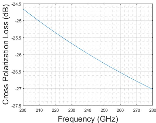
Fig. 4 Cross polarization loss as function of the frequency. The frequency range spans that cover by Band 6. The loss has a value of -26 dB at the central point.
