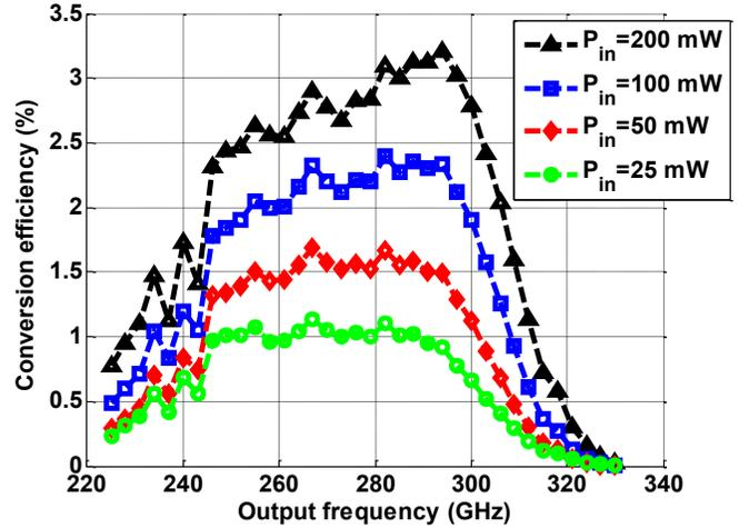
Fig. 3. 300 GHz frequency tripler: conversion efficiency as a function of output frequency for the 25-200 mW input power range.
