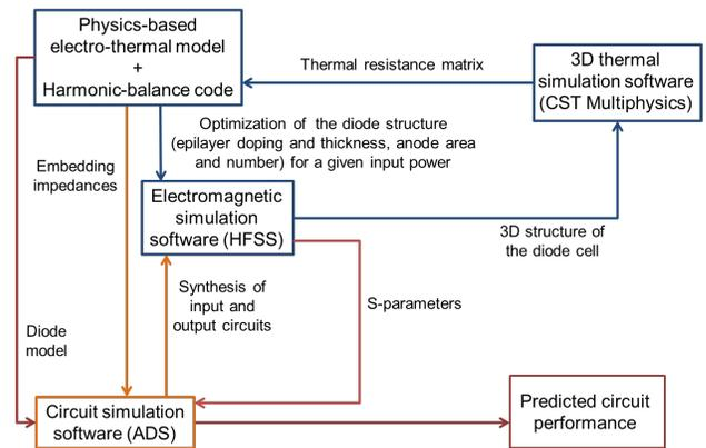
Fig. 1. Iterative design process utilized to optimize circuit performance.
