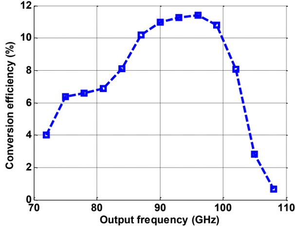
Fig. 2. 94 GHz frequency tripler: conversion efficiency as a function of output frequency for an input power of 100 mW.
