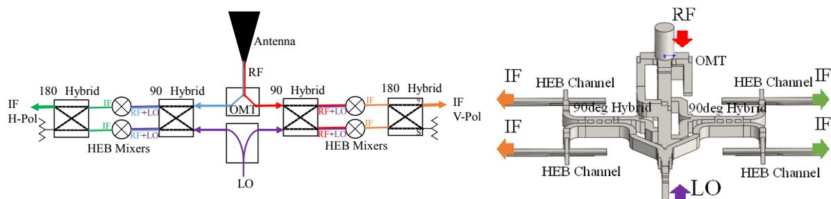
**Figure 1:** (a) Block diagram and (b) actual waveguide design of the dual-polarized, balanced receiver front-end at 1.9 THz fabricated with silicon micro-machining technology.
