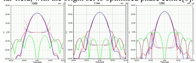
Fig. 1 Improved diagonal horn simulation for three frequencies. X-pol (45°) is in green. Ludwigs 3<sup>rd</sup> definition of cross-polarization[8] is used.
