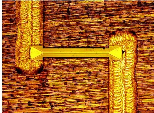
*Fig. 1 A view of the microstrip-to-waveguide probe chip as installed in the E-plane split block. Also visible are the WR3.4 waveguides each with a single capacitive tuning step.*
