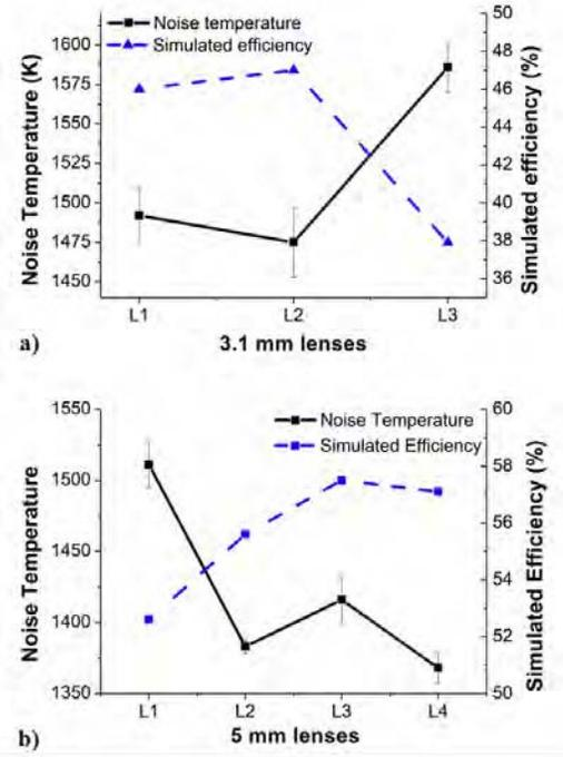
Fig. 4. Noise temperature measurements and PILRAP efficiency simulations. a) 3.1 mm lenses. b) 5 mm lenses.
