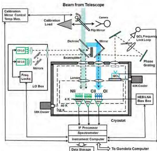
Fig. 1 GUSTO instrument block diagram, which was in the original proposal. It is still in progress with regard to, in particular, the 4.7 THz LO.
