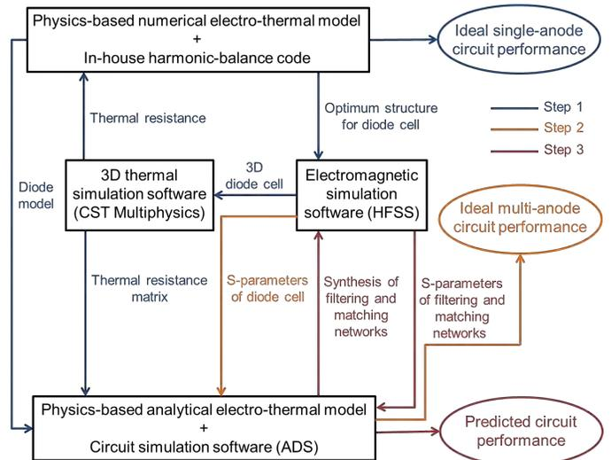
Fig. 1. Iterative design process utilized to optimize circuit performance.
