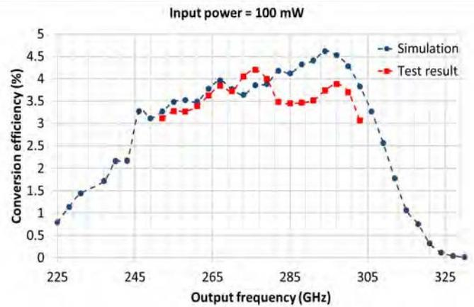
Fig. 3. 225-315 GHz frequency tripler: Conversion efficiency as a function of output frequency for an input power of 100 mW.
