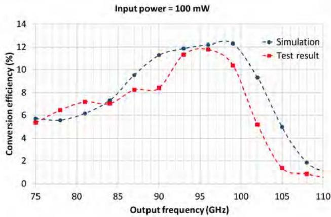
Fig. 2. 75-105 GHz frequency tripler: Conversion efficiency as a function of output frequency for an input power of 100 mW.
