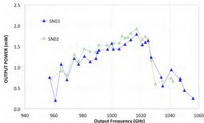
Fig. 3: A compact 1 THz LO chain has been built and demonstrated. The measured power should be sufficient to pump Schottky diode mixers in the 2 THz range.
