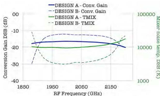
Fig. 2 Simulated performance of the two mixer chips as a function of frequency is shown. Identical anode parameters are selected for both designs.
