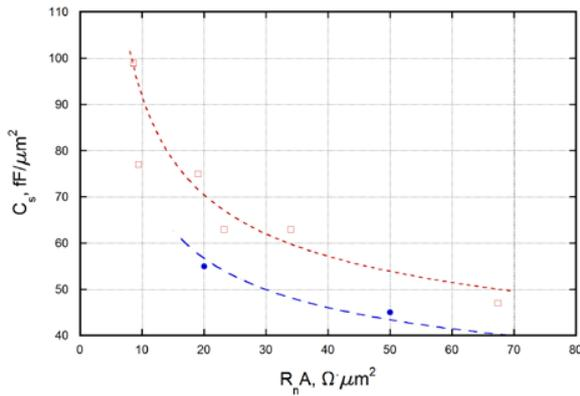
Fig. 5. Specific capacitance of Nb/Al-AlN/Nb junction (red) as compared with that of Nb/Al-AlO<sub>x</sub>/Nb junctions [5] (blue). The capacitance data for the junctions are approximated with empirical relation  $C_s = a/\ln(R_nA)$  [14], where  $a$  is equal to 211 [5] for the Nb/Al-AlO<sub>x</sub>/Nb junctions and to 170 for the measured Nb/Al-AlN/Nb junctions.
