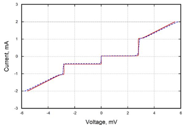
Fig. 3. Comparison of an Nb/Al-AIN/Nb junction as fabricated (red) and after annealing sequence up to 200°C (Fig. 2).
