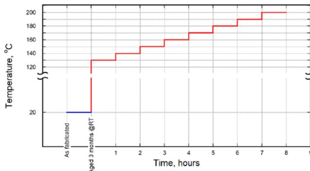
Fig. 2. Temperature profile of aging/annealing of AIN-barrier junctions [2].
