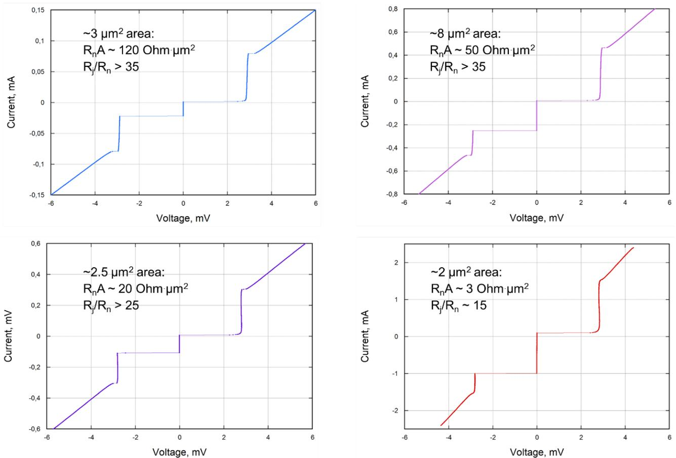
Fig. 1. Examples of Nb/Al-AIN/Nb junctions' current voltage characteristics with  $R_n A$  ranging between 3 and 120  $\Omega \cdot \mu\text{m}^2$ . The legend inside each plot panel shows junction's size,  $R_n A$  and  $R_j/R_n$  values.
