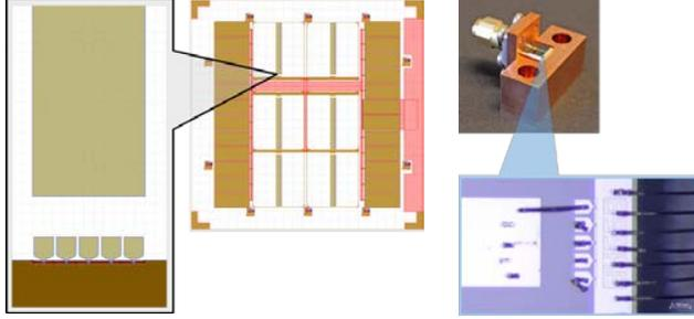
Fig. 4. The test junction wafer containing 20 single junctions of the sizes 3, 4, 5, 6 and 8  $\mu\text{m}^2$  connected to the external contact pads. The six chips for measurement of specific capacitance each have 50 $\Omega$  line and single junctions of the sizes 3, 4, 5, 6 and 8  $\mu\text{m}^2$  to be connected by bonding.
