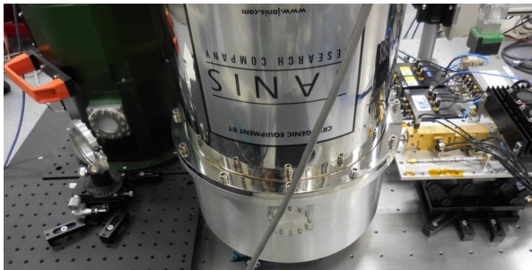
Fig.4. Photograph of measurement set up of receiver noise temperature of the Ni-NbN HEBM. The LO signal was taken out from the cryostat and reflected by a polyester beam splitter (BS) with a thickness of 4 \mu\text{m} of which the reflection coefficient is \sim 5\% , and was fed into an HEBM cooled by another LHe dewar. As a first step experiment, the BS and HEBM were put outside the cryostat because alignment is difficult inside the cryostat at the high frequency.
