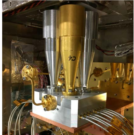
Fig. 1. Photo of the 4-beam mixer holder mounted inside the testing cryostat. Signals of 2 mm wavelengths are coupled through four corrugated horns attached at the upper side. The single LO injection port is seen at the near-side of the block. IF/DC are conducted by using 16 coaxial cables.
