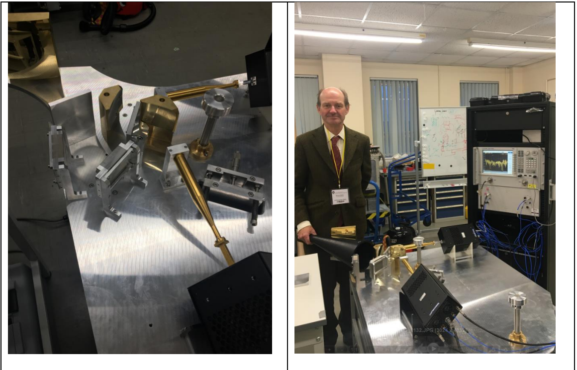
Figure 4: GRaCE 200 GHz quasi-optical multiplexer close up (left) and under VNA test at RAL with Dr Richard Wyld of TK Ltd. (right).
