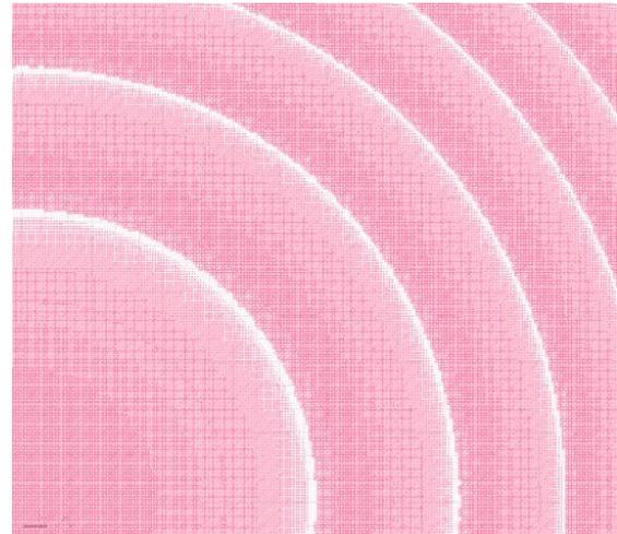
Fig. 1. A zoomed-in image of a single layer of the lens manufacturing drawing. Each pink square will be a conductive element embedded in polyimide.
