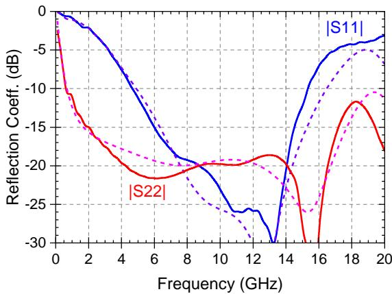
Fig. 3. Measured (solid lines) and simulated (dashed lines) input and output reflection of the LNA at 15 K ambient.
