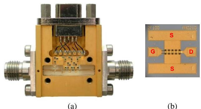
Fig. 1. (a) Photograph of the three-stage 2-18 GHz CLNA without cover. Dimensions excluding connectors are 20x22x9 mm. (b) 2x100  $\mu\text{m}$  gate finger InP HEMT in 100 nm technology used in the 1<sup>st</sup> stage of the amplifier.
