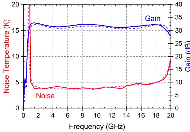
Fig. 2. Measured (solid lines) and simulated (dashed lines) gain and noise temperature of the LNA at 6 K ambient.
