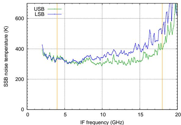
Fig. 5: The noise temperature for both sidebands at the same LO frequency as fig. 4. Note that this is the single-sideband (SSB), which is intrinsically double that of the individual DSB mixers, even any added components are lossless).
