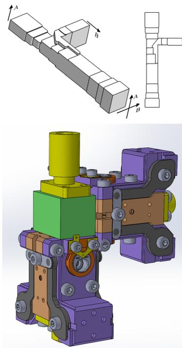
Fig. 6: Top: structure of the OMT by Dunning et al. (image from [18]). Bottom: the basic geometry of two SEPIA660-type Band 9 2SB mixers around a block (green) that could contain a Dunning-type OMT. The OMT structure itself will be about 2 mm long in the Band 9 frequency range and will certainly fit in a block like this.
