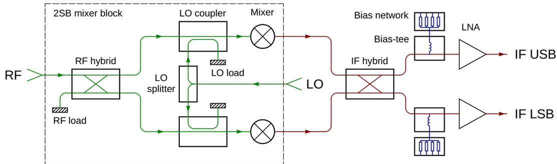
Fig. 1: Schematic diagram of the classical 2SB mixer architecture used in the study (as well as in the SEPIA/LLAMA receivers). Waveguides in green, IF coaxial cables/strip lines in red, DC lines in blue. Each “Mixer” denotes a single-ended (DSB) SIS device. A full receiver typically contains two such assemblies, for orthogonal polarizations. Further details in [8].
