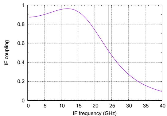
Fig. 2: Simulated IF power coupling of the Band 9 SIS junction at the operating point.
