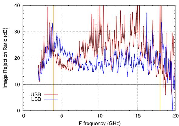
Fig. 4: The IRR singled out for one LO frequency near the middle of the band (662 GHz) over the full 2–20 GHz IF band. The vertical yellow lines indicate a usable band of 4–18 GHz.
