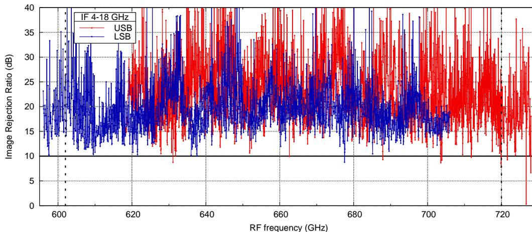
Fig. 3: The combined IRR data for the tested 2SB mixer with ultra-wide band IF infrastructure and 8 GHz-spaced LO settings, as function of the RF frequency. The IF range of each sub-trace is limited to 4–18 GHz. The horizontal black line at 10 dB indicates a typical specification of similar receivers.
