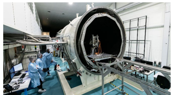
Fig. 2 Testing of SWI inside the LORENTZ chamber
