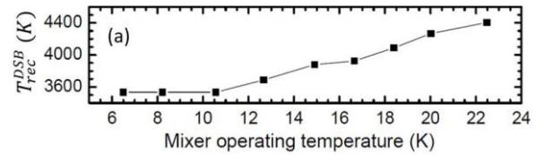
Fig. 1. Receiver noise temperature versus operating temperature
