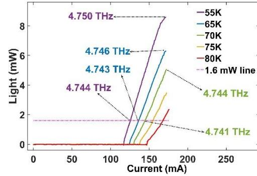
Fig. 1. Light-Current with measured frequencies indicated in the inset.
