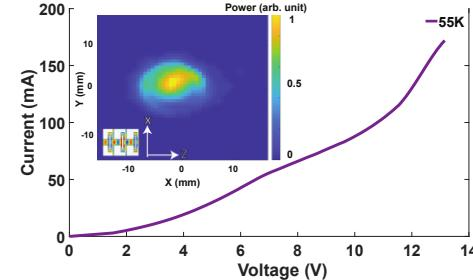
Fig. 2. Measured Voltage-Current and beam pattern as inset.
