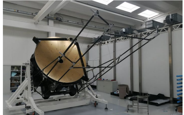
Fig. 1. ASTHROS payload under I&T, showing the 2.5-m primary mirror and the \sim 4.5-m long sunshade frame,
