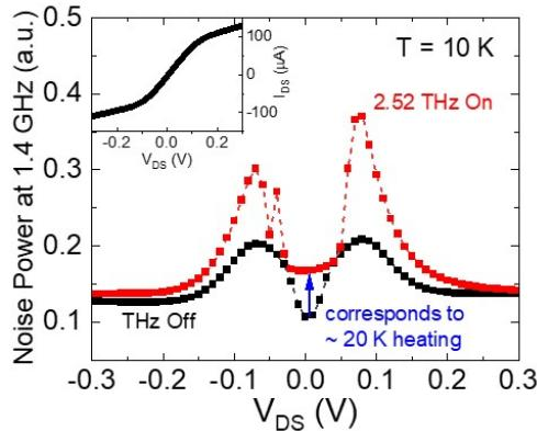
Fig. 2. DC-bias dependence of the noise power at 1.4 GHz with and without 2.52 THz at 10 K. The inset shows the device current-voltage (IV) curve without THz illumination at 10 K.
