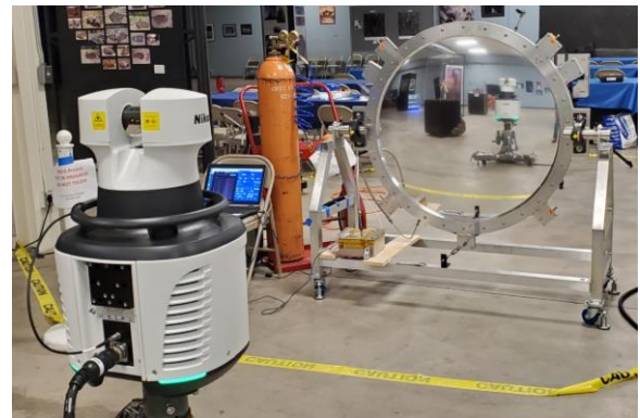
Fig.2 Nikon APDIS laser radar measuring the surface profile of 1m A1 prototype.
