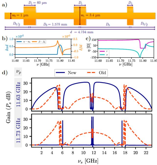
Fig. 1 (a) Unit cell of the used Floquet TL. (b) Dispersion relation near the 2<sup>nd</sup> stopband, where  $\gamma_0 = \alpha_0 + j\beta_0$  is the propagation constant of the central line. (c) Complex impedance near the 2<sup>nd</sup> stopband. (d) Gain of the signal after traveling  $z/d = 150$  unit cells for two values of pump frequency  $\nu_p$  near the 2<sup>nd</sup> stopband, using an initial pump amplitude  $A_p^0 = 0.2 I_*$ .
