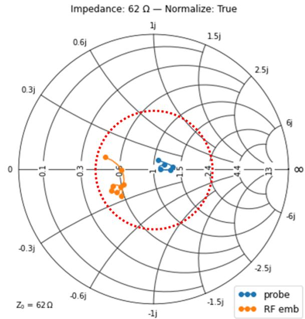
Fig. 3. The power from the feed point is transferred to the junction through tuning elements and it is finally seen to the junction as an RF embedding impedance. The RF embedding impedance of the Type 1 circuit from RF 211 to 275 GHz is located inside of the  $|\rho| = 0.4$  circle indicated as a red dashed line. The Smith chart is normalized with an optimum source impedance.
