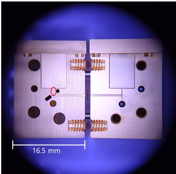
Fig. 2. Photo of the top and the bottom block of the mixer block (from left to right). The WR3.7 input waveguide is seen at the center. The mixer chip will be placed in the red-circled slot.
