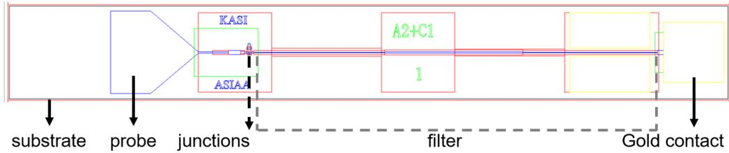
Fig. 4. The configuration of the mixer chip. The layers are denoted in different colors and the number in the center is information about the circuit and the number of columns on the wafer. The largest rectangle on the edge is a substrate. The probe at the left is a connection between the waveguide to the thin-film microstrip. The bonding pad is located at the last section of the RF choke followed by a gold contact. The gray dotted line is indicating a range of the RF filter composed of CPWs.
