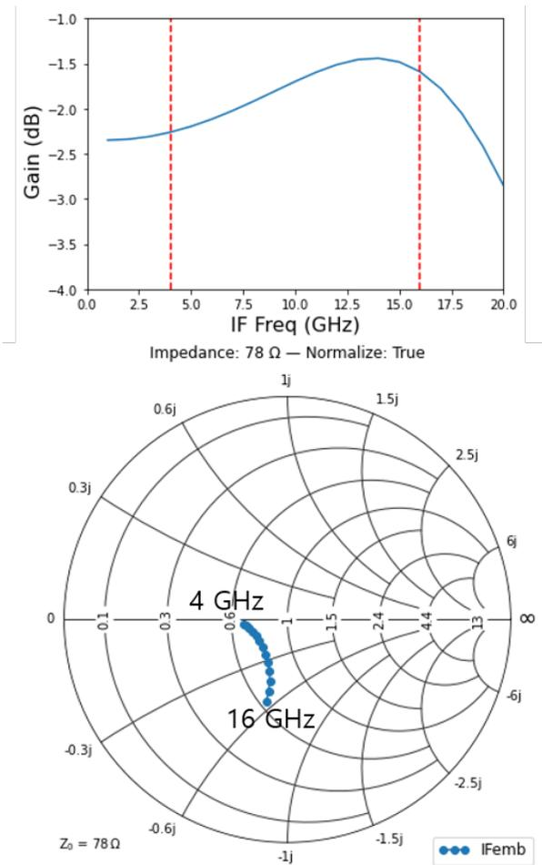
Fig. 7. The gain curve and IF embedding impedance of Type 1 from IF frequency 4 to 16 GHz with LO 243 GHz, which is normalized to 3 times of  $R_N$ . The gain curve has a peak at 14 GHz and the IF embedding impedance has the largest real part at the same point. It replies that the change of the gain is mainly contributed by the matching between the if impedance of the junction and the real part of the if embedding impedance.
