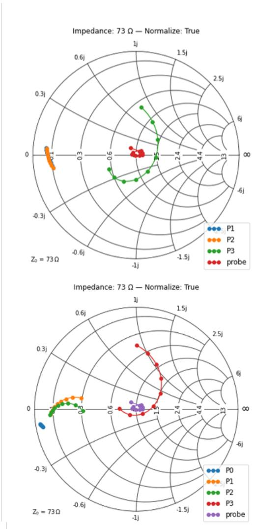
Fig. 5. (Top) An enlarged view of the Type 1 circuit between the probe and an island where the junctions are located. Thick lines are indicating the respective planes where the impedances are obtained. We can see the impedance is matched to the probe impedance from P1 to P3 through tuning elements. (Bottom) A maximized view of a Type 2 circuit showing an impedance matching from P0 to P3 through microstrips and CPWs.
