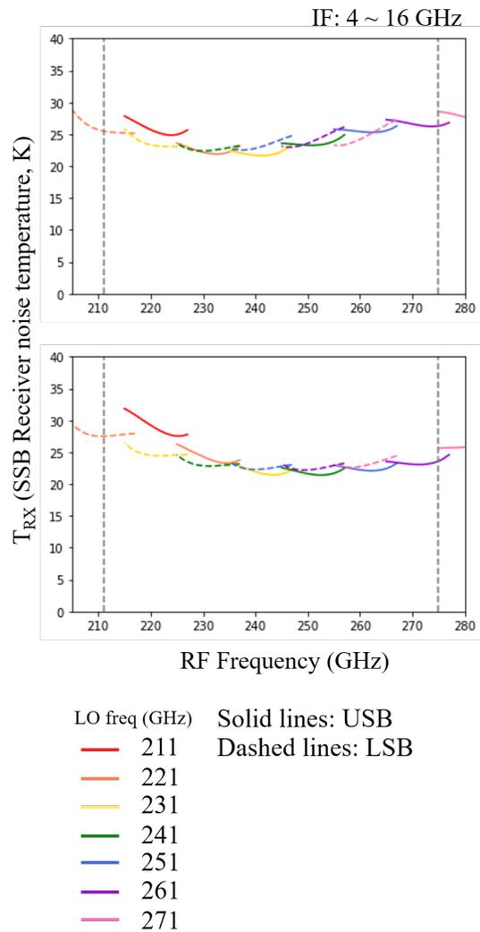
Fig. 6. The performance of designs simulated in Supermix. The top is for Type 1 and the bottom is about Type 2.  $T_{RX}$  is an SSB noise temperature and is calculated using a gain and a mixer noise temperature. Solid lines denoted upper sideband (USB) receiver noise temperatures with specific LO frequencies from 211 to 271 GHz and dashed lines are for lower sidebands (LSB).
