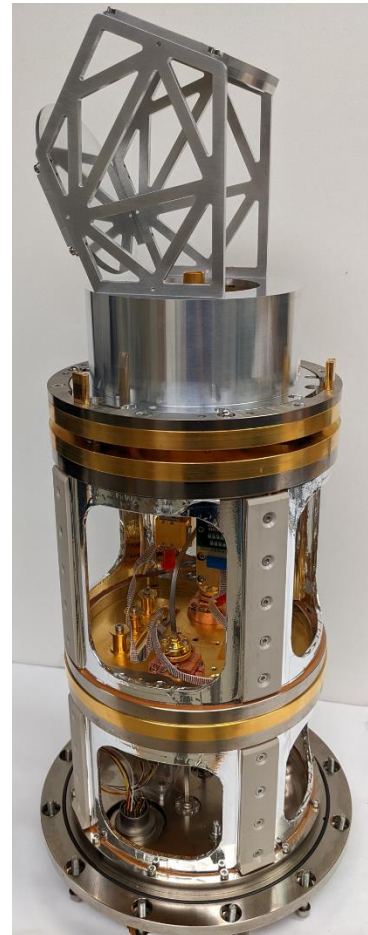
Fig. 1. Photo of a wSMA receiver cartridge. The upper section comprises the receiver optics, coupling the signals from the cryostat optics to the frontend assembly located inside the base of the receiver optics. The 4K plate is divided into a floating-4K and a fixed-4K stage for optical alignment purposes. The image also shows the 50K plate, the lower 300K plate, and the G10 shells providing support between the stages.
