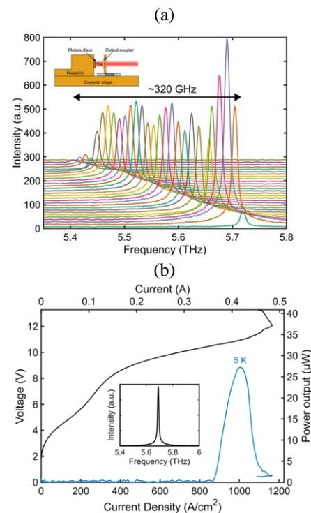
**Fig. 3.** (a) Stacked spectra of the QC-VECSEL output collected via FTIR that demonstrates single-mode tuning over a 320 GHz bandwidth. The spectra were collected in pulsed mode at 5 K. The inset shows a diagram of the VECSEL configuration, where the output coupler is mounted on a piezoelectric stepper motor to step the cavity length intra-cryostat (b) Power-current-voltage plot of the QC-VECSEL operating at 5.69 THz in pulsed mode.
