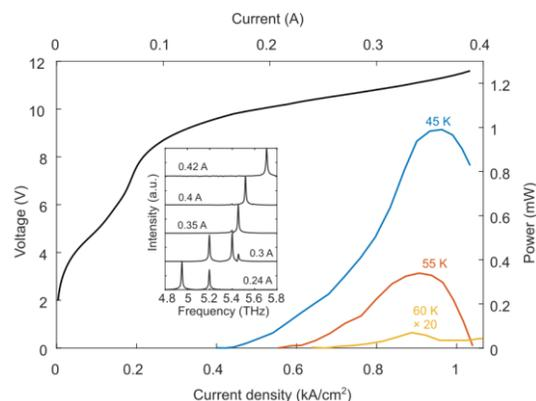
**Fig. 1.** Power-current-voltage data for a 0.5 mm x 75  $\mu\text{m}$  metal-metal waveguide operating in continuous-wave mode at various heatsink temperatures. The inset shows the measured spectrum from an FTIR at various bias points, with modes spanning from 4.95 to 5.71 THz.
