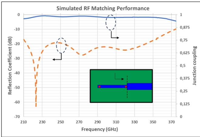
Fig. 2. Simulated performance of the RF matching circuit. For the HFSS simulation a lumped port was located as illustrated by the miniature. The impedance values for the twin junction circuit were calculated and load in the lumped port.
