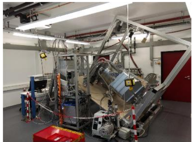
Fig. 1. The AMKID instrument installed in the laboratory test system. The setup allows to tilt the instrument to its normal operation conditions. A large Liquid Nitrogen load provides a background loading similar to the expected atmosphere load.
