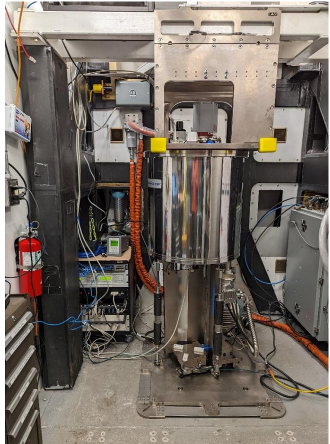
Fig. 1. Photo of the prototype wSMA receiver installed in SMA Antenna 7.
