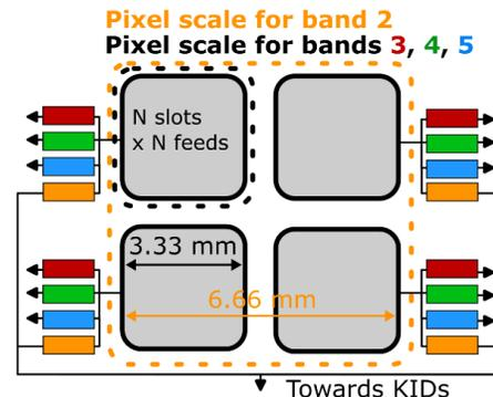
**Fig. 1.** Schematic of the hierarchical phased-array antennas. The  $N$  slots of each pixel are coherently summed using microstriplines. Each pixel is connected to lumped-element band-pass filters corresponding to bands 3, 4, and 5, while the four pixels are coherently summed together and connected to the band-pass filters defining band 2.
