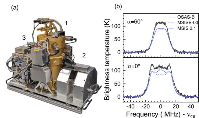
**Fig. 1:** (a) Photograph of the instrument. 1: cryostat, 2: optics compartment, 3: backend electronics. (b) Measured and simulated spectra for 60° and 0° elevation. Observation: 2022/09/07 9:14 UTC, 68°19'N, 19°40' E, height: 32.6 km, azimuth direction: 23° NNE. Simulated spectra based on the NRL MSISE-00 [3] and MSIS 2.1 model [4].
