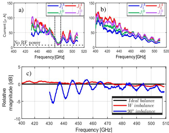
**Figure 4:** Measured current at constant  $V_{bias}=1.8$  mV of the 4 SIS junctions of the 2 balanced mixers in the 2-pixel block while sweeping the local oscillator over the frequency band and deducted power division balance of the power dividers (a) 90° hybrid power divider. (b) Wilkinson power divider. (c) Balance of the power dividers, here  $J_1$  of both mixers A and B is compared, effectively yielding the amplitude imbalance of the power divider.
