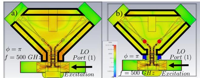
**Figure 6:** 3D simulation of IBAMI in its housing cavity, the beamlead pocket footprints is highlighted in the black outline. (a) Field simulation at  $f = 500$  GHz in the original cavity. (b) Field simulation at  $f = 500$  GHz in the modified cavity.
