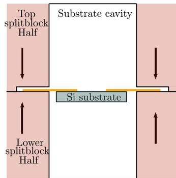
**Figure 7:** Cross-section of the housing cavity of the IBAMI with beamlead pockets depicted. These pockets are milled over the beamleads to prevent mechanical degradation from several open/close cycles of the block.
