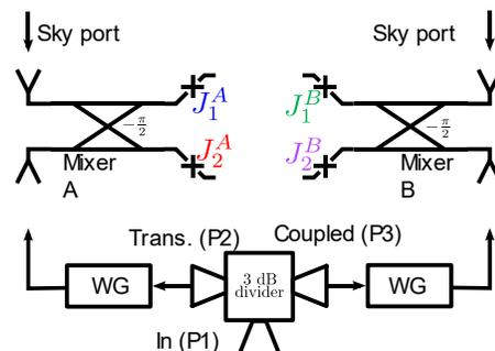
Fig. 2. Schematic of the 2-pixel block with the two mixers and power divider connected by the long waveguide.
