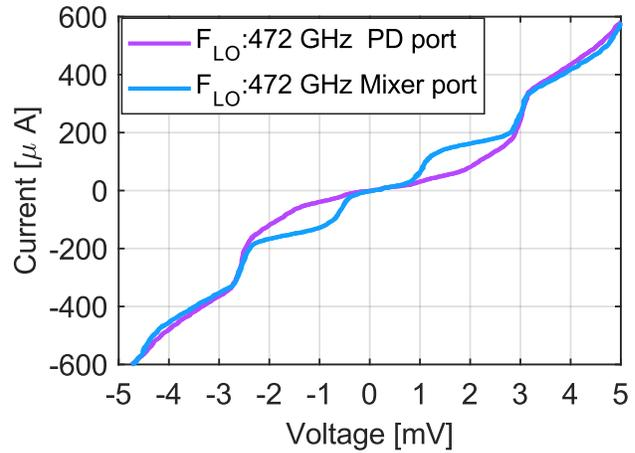
**Figure 5:** I-V characteristics of the SIS junctions with RF power coupled through the power divider (violet curve) and the horn (blue curve) for the same junction.
