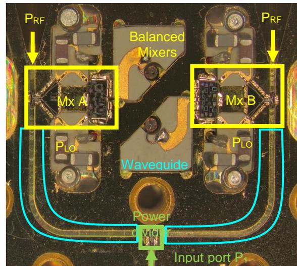
Figure 1: Microscope photo of the populated 2-pixel block's lower half.
