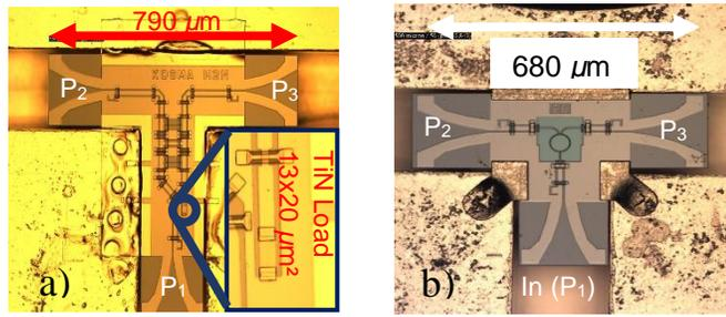
**Figure 3:** Microscope photos of the 2-pixel block and both power dividers. a) Bottom half of the populated w-pixel block. b) 90° three branch line CPW power divider, terminated with a resistive load c) Wilkinson power divider
