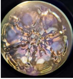
Fig. 6. Optical micrograph of the prototype at 1.627 THz manufactured via diamond machining at Fraunhofer IOF (Jena, Germany).
