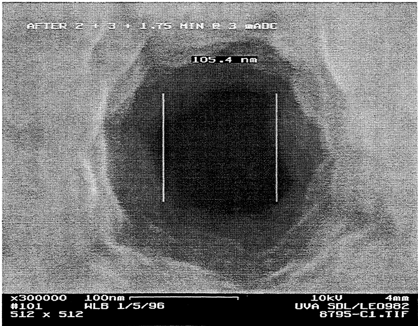
Fig. 5. Anode pattern after electroplate window shrink (EWS)
